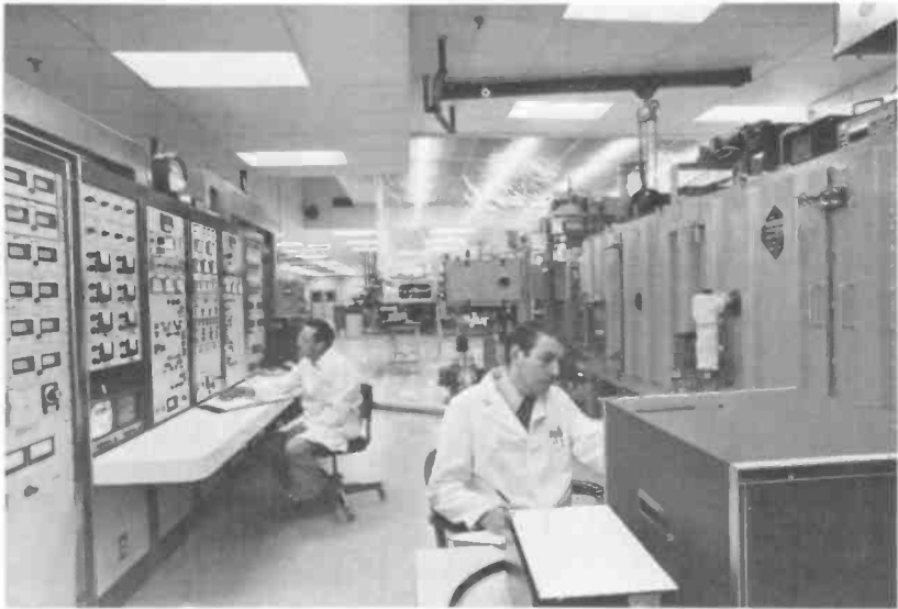
Fig. 5—(A) View of the "back" side of the coater showing the four turbomolecular pumps. (B) View of the "front" side. A mass spectrometer head is attached to a port in the dielectric chamber. The control panels for the coater are seen at the left.
