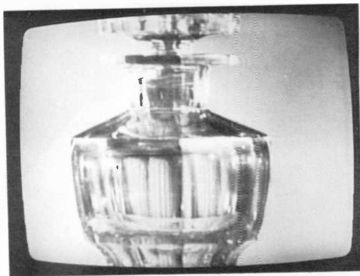
Fig. 7—Photograph of a picture reproduced on a TV screen while playing from a one-hour-per side disc.
