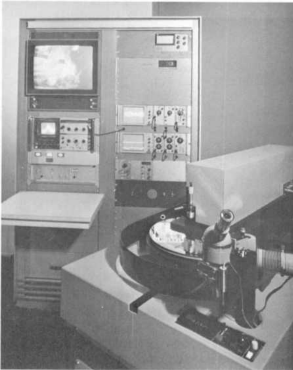
Fig. 9—Photograph of a VideoDisc optical reading system developed for routine production control.
