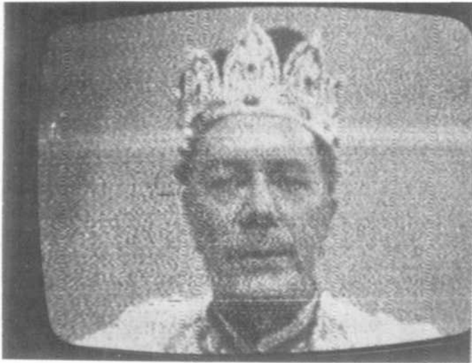
Fig. 2—Photograph of picture reproduced on a TV screen while playing a disc made from an early (July 1971) electron-beam recording.
