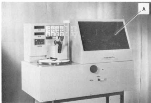
Fig. 13—Photograph of a defect detector developed for routine production control (A is the fully interlocked cover for the laser system).
